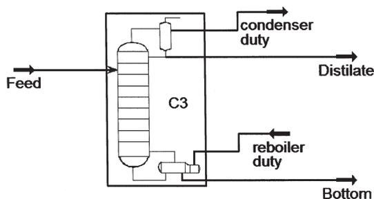
Fig. 4. Steady-state simulation diagram for propylene-propane distillation column
