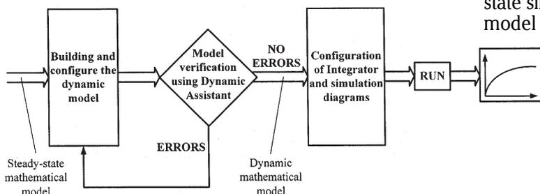
Fig. 3. Detailing the development of dynamic model
