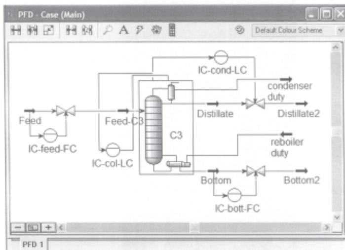
Fig. 9. Dynamic simulation diagram of the distillation column
