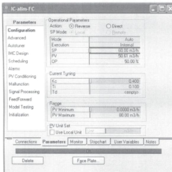
Fig. 10. Change of set point for feed flow rate control system
