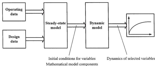
Fig. 1. Structure of operations associated to dynamic simulation
