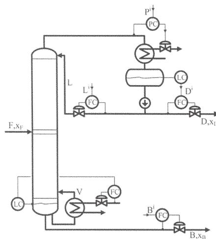
Fig. 8. L-B control structure
